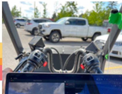
OAK1-Lite: Testing other mounting positions for the cameras (green tape on the right).
